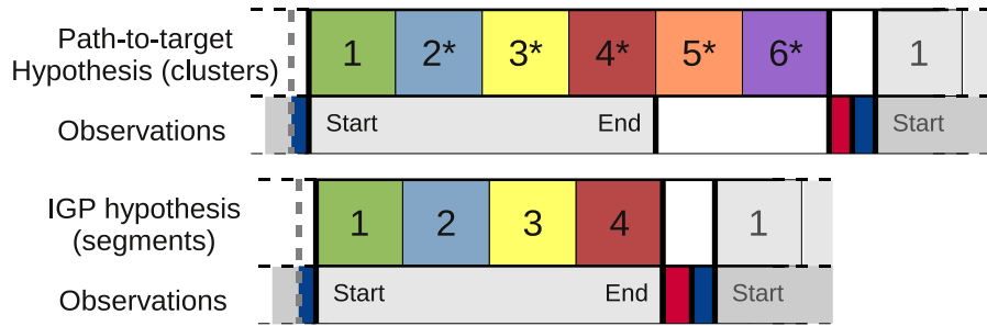
Figure 5.16: Timing diagram showing the number of parameters for the path-to-target and the IGP hypotheses and how they compare to the observation time. The IGP parameters are fixed to 4 segments, whereas the path-to-target clusters the targets, resulting in 1–6 parameters, depending on the number of clusters chosen (*optional). If there are 4 or fewer clusters then the observation timing becomes the same as IGP.
