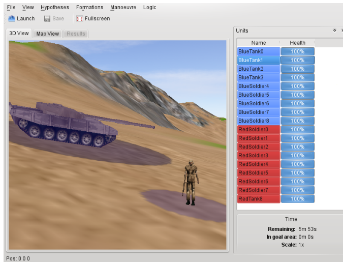
Figure 4.5: Simulator screenshot. This shows the interface for the human-controlled teams. The main 3D view is used to issue commands to the units. The status of each unit is shown in a panel on the right of the screen. The tabs allow the user to access a 2D map of the unit positions and their predicted movements.
